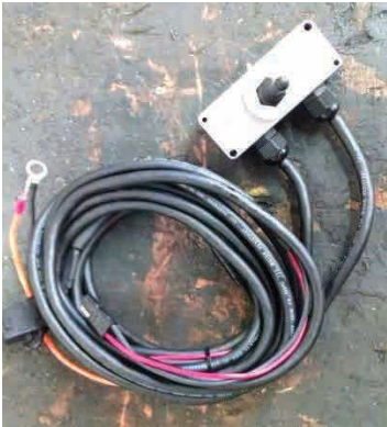
Connect Wire Harness on Model with Hydraulic Angle (only)
