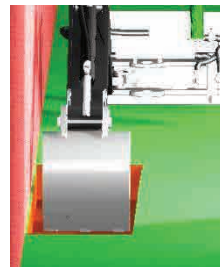
Back in Offset Position, Excavating next to wall
