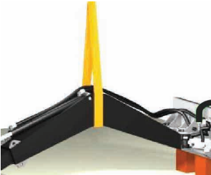
Supporting Boom during Conversion
